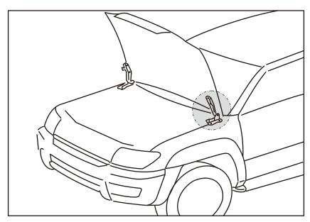
**2**. Loosen bonnet car hinge nuts at the passenger side, but it doesn't come loose.
