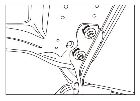
. Locate the aerial mount between the two nuts.
